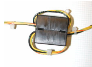
closed ferrite core, triple wrap
