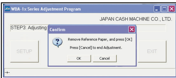
Figure 6-14 Remove Calibration Paper Screen Calibration with White and Black Paper is now complete. Remove the final calibration paper and close the Acceptor Head (See Figure 6-15 a). Make sure that the tabs on both side of the Acceptor Head are once again firmly locked in place (See Figure 6-15 b).
